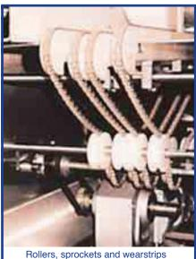
manufactured from TIVAR® H.O.T. for applications in food processing show no signs of wear after numerous chemical and water washdowns, unlike their stainless steel counterparts.
